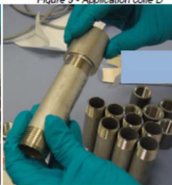
Figure 11 - Assemblage colle D
