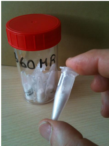
Figure 6: Microcentrifuge tube filled with a MN sample of 0.5 cm 3 for a dustiness test according to the VS method.
