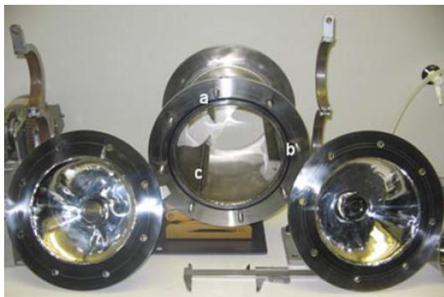
Figure 1 : Photograph showing the high-gloss polished inside of the dustiness drum. Also note the three lifter vanes marked a, b, and c at each 120° in the drum.
