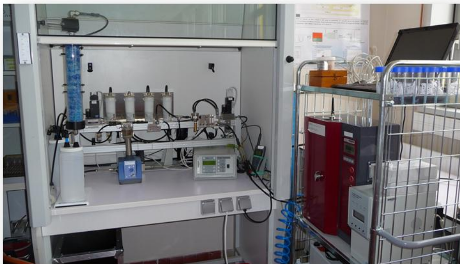
Figure 7 : Overview of the vortex shaker set-up positioned in the variable flow fume hood at INRS.
