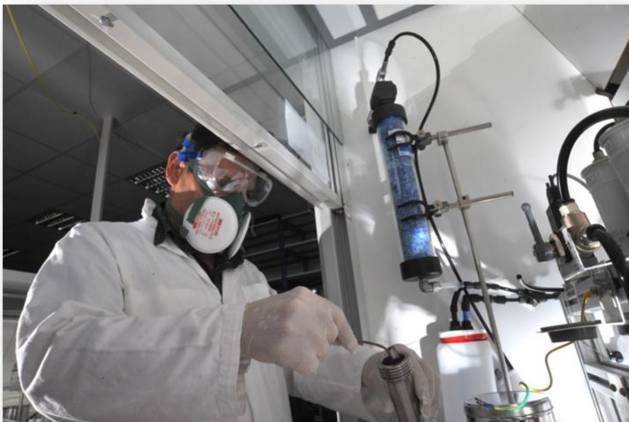
Figure 10: Operator introducing a MN sample into the Vortex Shaker positioned in the variable volume fume hood used at INRS.
