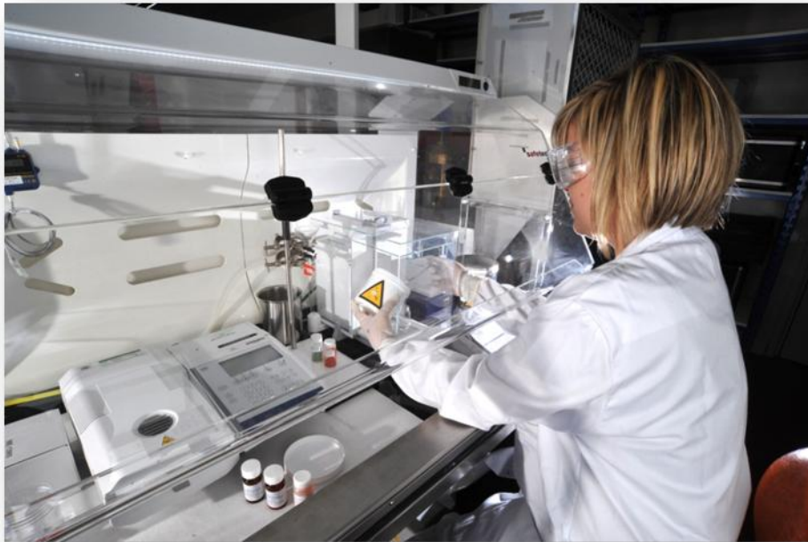
Figure 9 : Operator during MN sample preparation (weighing and water content measurement) in the powder handling enclosure at INRS.
